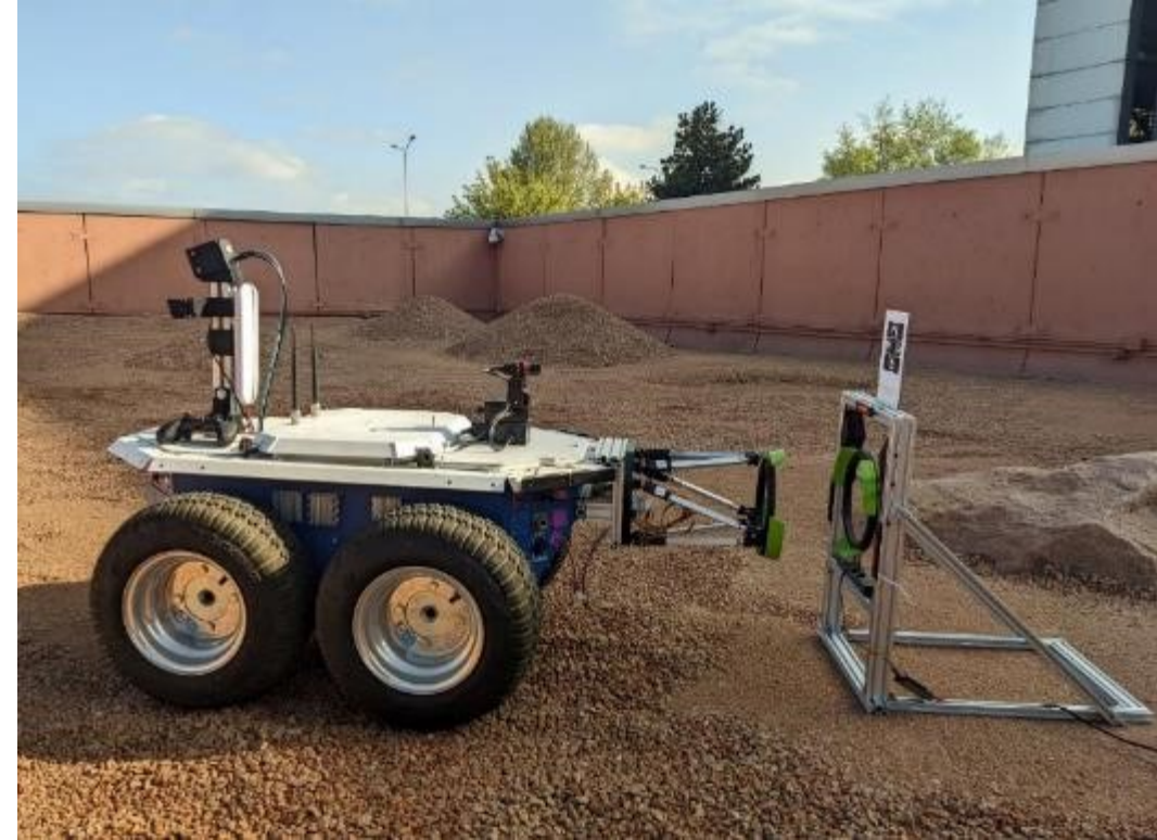
Advanced fully Autonomous Navigation (localization, mapping, planning), autonomous docking of surface elements through vision systems – Completed, to be deployed on more advanced systems
